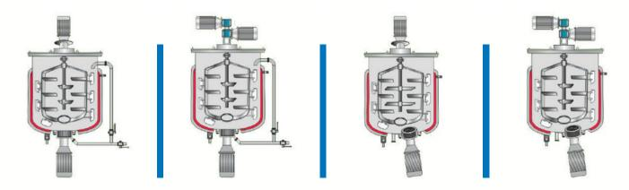
Single way mixing & external circulation Double way mixing & external circulation Single way mixing & internal circulation Double way mixing & internal circulation
